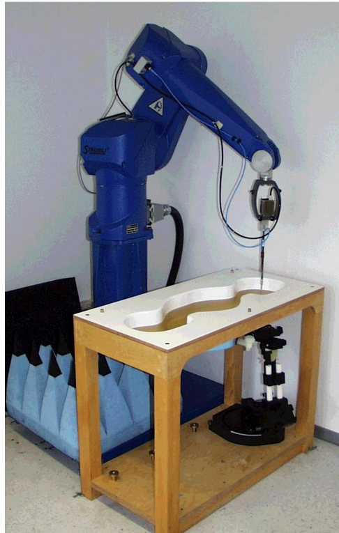
Fig. 7: The measurement setup with a phantom containing tissue simulating liquid and a device under test.
