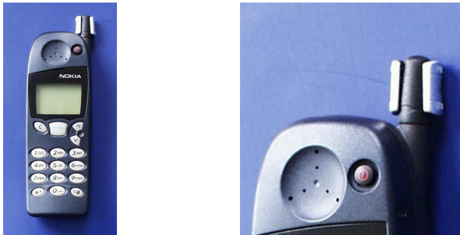
Fig. 1: Pictures of a Nokia 5110 with the SAR SHIELD accessory.
